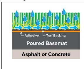
Water runs horizontally across top of turf backing at minimum 2% slope toward low end(s) to perimeter curb(s) with weep holes, open fence, or sloped edge.
