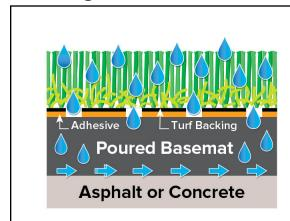
Water runs through 1/4" diameter perforations in turf backing and adhesive (as shown) into porous basemat. Water then migrates to bottom of basemat and runs horizontally with slope of asphalt or concrete to one or more drainage basins under the basemat.
