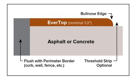
**Drainage:** Water both sheds off top of the surface and penetrates the surface and runs horizontally through the material with the slope of the asphalt or concrete toward the low end(s).
